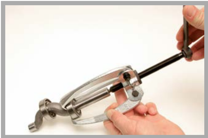
Disassembly of the piston pump: pulling off the ball bearing of the eccentric shaft (using a bearing puller)
