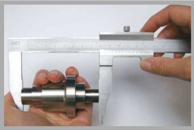
Measurement of length using a caliper gauge
