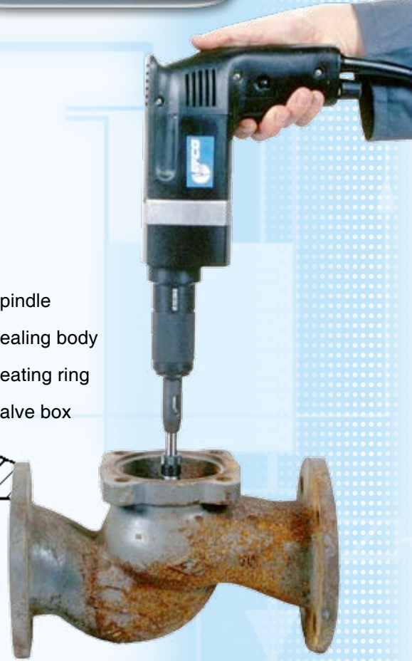
Grinding of the seat of a flatseat valve
