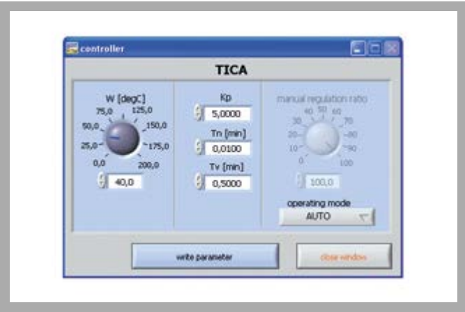
Controller operation via process schematic: reference variable, controller parameters and controller mode (manual or automatic) selectable
