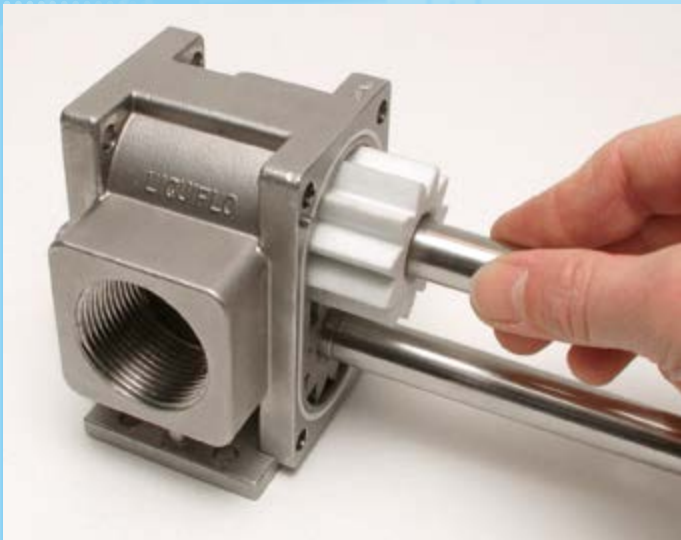
Installing the driven shaft
