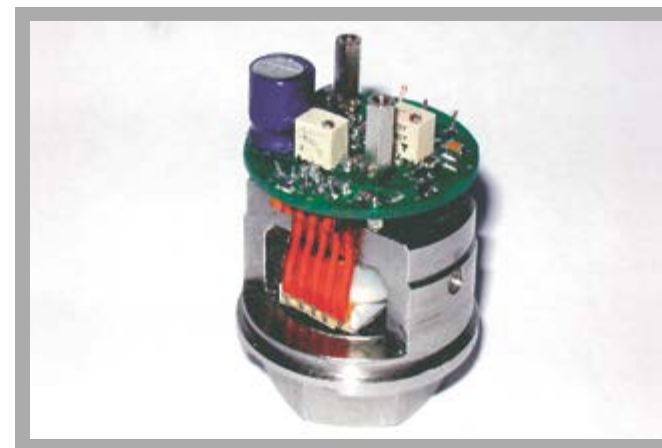
Interior layout of an electronic pressure sensor
