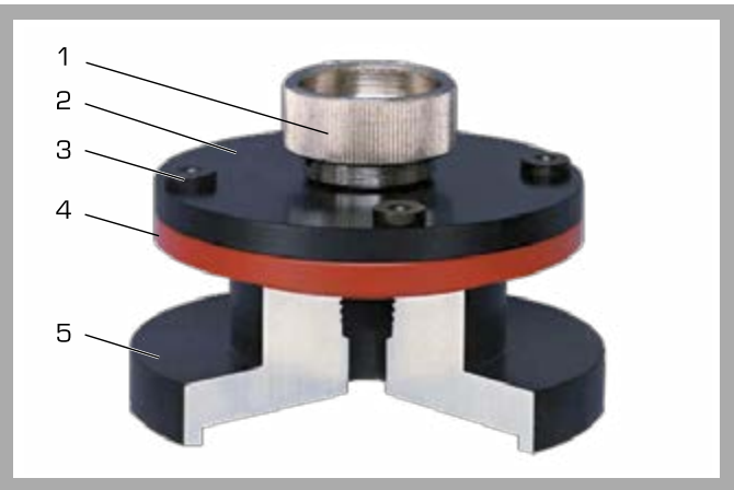
Assembled drilling jig with workpiece: 1 fastening screw, 2 drilling plate, 3 drill bush, 4 workpiece (bearing cover), 5 main drilling jig body
