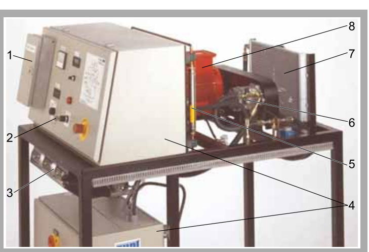
1 box with fault buttons, 2 ignition key, 3 air cooler with three-stage fan, 4 switch cabinet, 5 flow meter, 6 compressor, 7 condenser with fan, 8 electric motor
