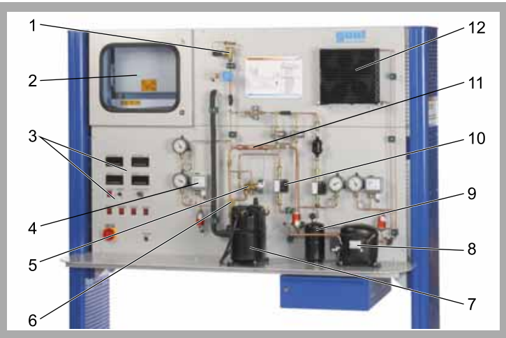
1 expansion valve, 2 refrigeration chamber, 3 displays and controls, 4 pressure switch, 5 injection valve, 6 injection cooler, 7 LP compressor, 8 HP compressor, 9 receiver, 10 flow meter, 11 heat exchanger, 12 condenser
