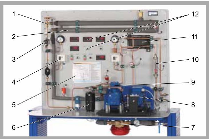
1 expansion valve, 2 evaporator, 3 refrigerant flow meter, 4 pressure switch, 5 process schematic, 6 receiver, 7 hot water circuit of the evaporator, 8 drive motor, 9 compressor, 10 cooling water flow meter, 11 condenser, 12 displays and controls
