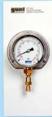
Component 10/03: Delivery side manometer
