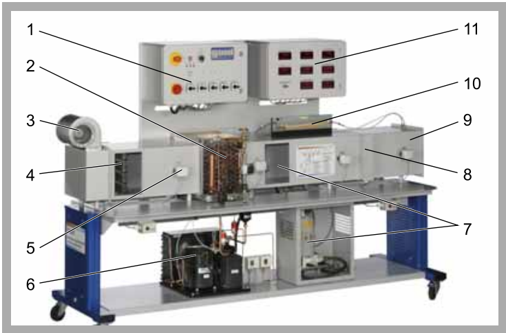
1 controls, 2 air cooler (direct evaporator), 3 fan, 4 air preheater, 5 temperature sensor, 6 condensing unit, 7 air humidifier, 8 air reheater, 9 air duct, 10 inclined tube manometer, 11 displays
