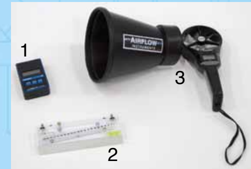
1 digital manometer, 2 inclined tube manometer, 3 anemometer
