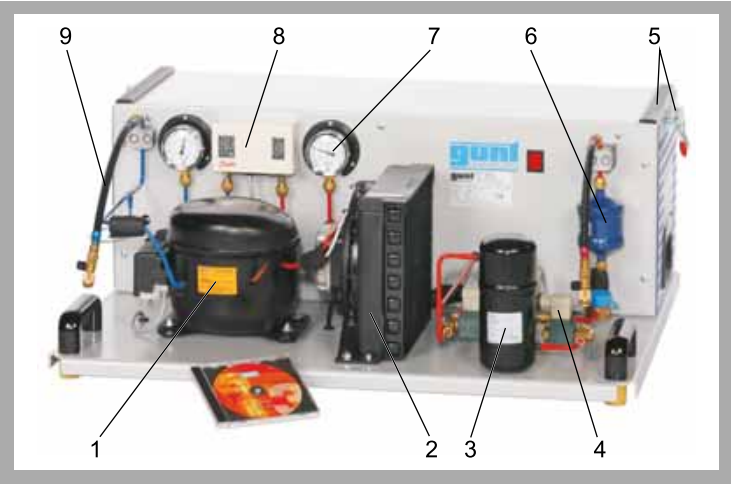
1 compressor, 2 condenser with add-on fan, 3 receiver, 4 solenoid valve, 5 frame to mount the models, 6 filter/drier, 7 manometer, 8 pressure switch, 9 refrigerant hose
