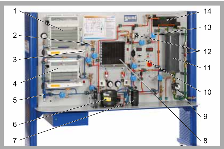
1 evaporator, 2 expansion valve, 3 capillary tube, 4 freezing stage evaporator, 5 evaporation pressure controller, 6 compressor, 7 receiver, 8 heat exchanger with fan, 9 pump, 10 display and control elements, 11 tank for glycol-water mixture, 12 flow meter, 13 solenoid valve, 14 coaxial coil heat exchanger
