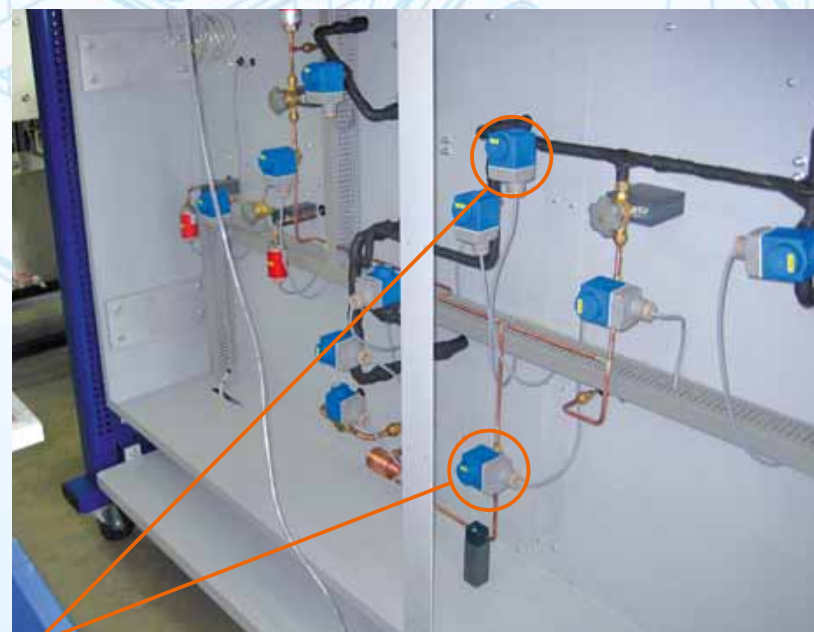
Solenoid valves at the back of the test stand to simulate mechanical faults
