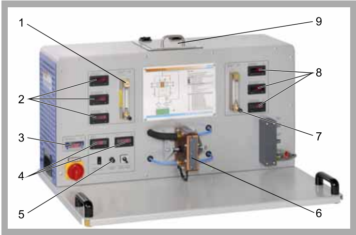
1 cold water flow meter, 2 temperature displays cold side, 3 water tank temperature controller, 4 voltage and current displays, 5 adjustment of the electrical power, 6 Peltier element with heat exchangers, 7 hot water flow meter, 8 temperature displays hot side, 9 water tank cover
