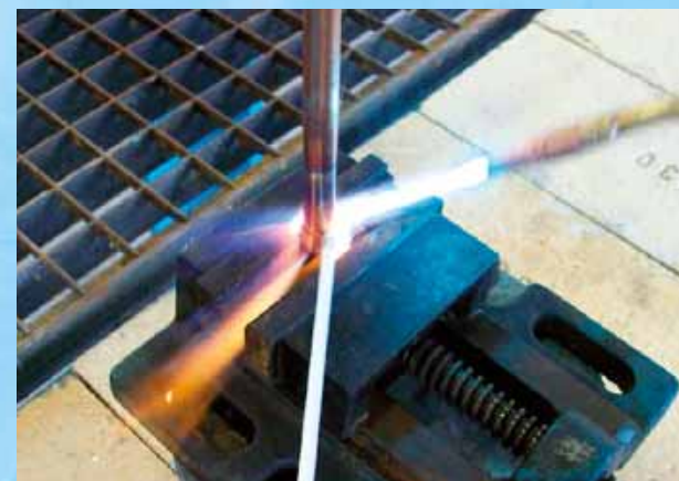
Heating the workpieces up to the soldering heat and melting of flux material and solder. By capillary effect solder automatically fills the soldering gap.
