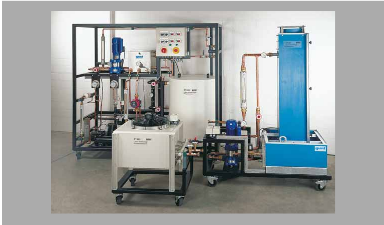
Trainer (in the background), dry cooling tower (in the foreground) and wet cooling tower (right)
