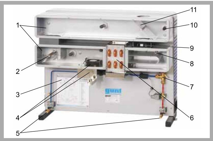
1 air duct, 2 air reheater, 3 process schematic, 4 air humidifier, 5 connections for ET 915, 6 evaporator, 7 expansion valve, 8 air preheater, 9 fan, 10 sensors for humidity and temperature, 11 ventilation flap
