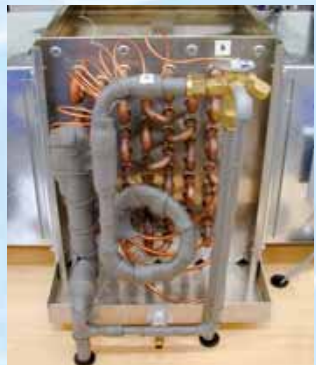
Direct evaporator as air cooler
