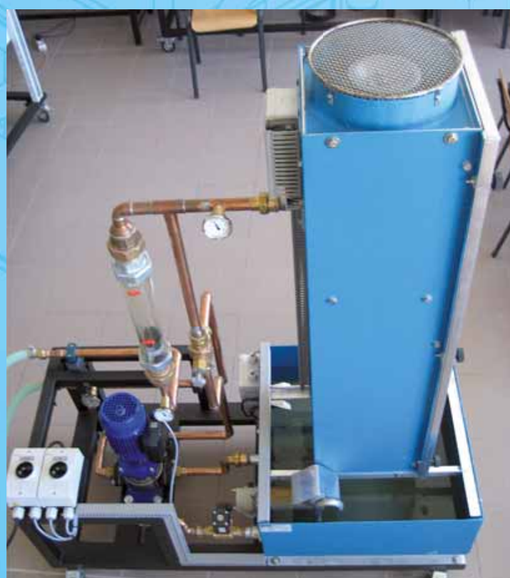
Plan view of the wet cooling tower
