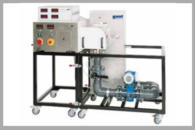
This picture shows a complete experimentation set-up: Axial-Flow Pump Module HM 365.45 connected to the Universal Drive and Brake Unit HM 365
