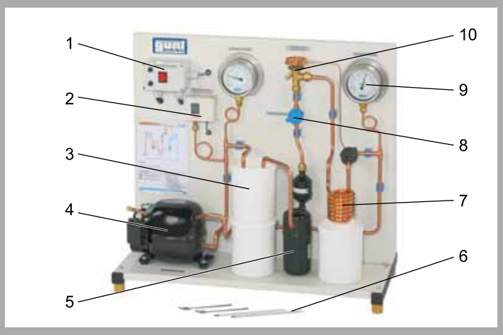
1 main switch, 2 pressure switch, 3 evaporator with water tank, 4 compressor, 5 receiver, 6 thermometer, 7 condenser, 8 sight glass (refrigerant), 9 manometer, 10 expansion valve
