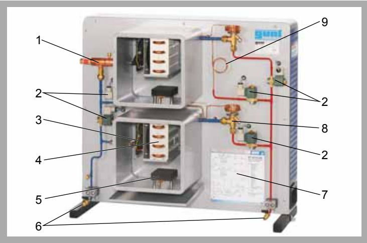
1 evaporation pressure controller, 2 solenoid valve, 3 fan, 4 evaporator, 5 heater, 6 connections to ET 915, 7 process schematic, 8 expansion valve, 9 capillary tube
