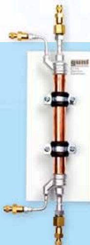
Component 10/06: Heat exchanger
