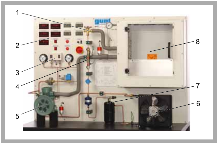
1 expansion valve, 2 displays and controls, 3 pressure switch, 4 flow meter, 5 compressor, 6 condenser, 7 receiver, 8 refrigeration chamber
