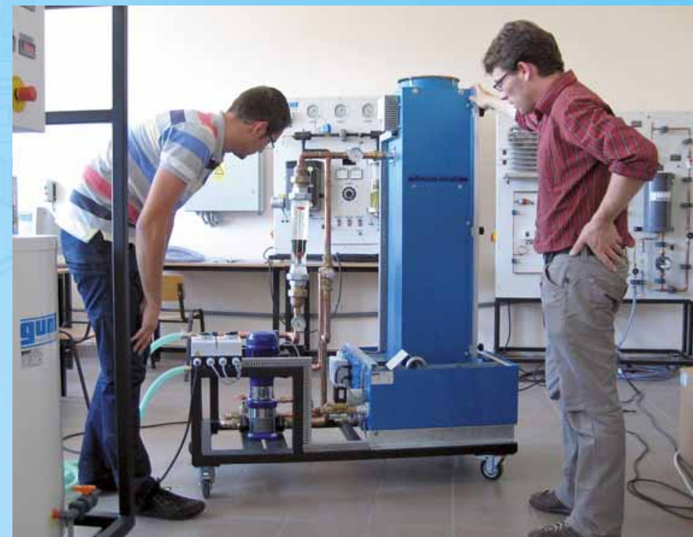
The wet cooling tower is connected and can be commissioned.
