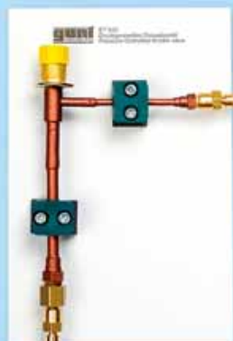
Component 10/07: Pressure- controlled expansion valve
