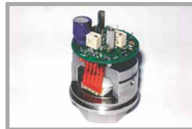
Interior layout of an electronic pressure sensor
