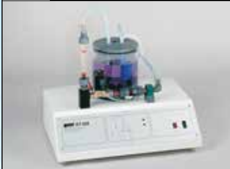
RT 030 Training System: Pressure Control, HSI
