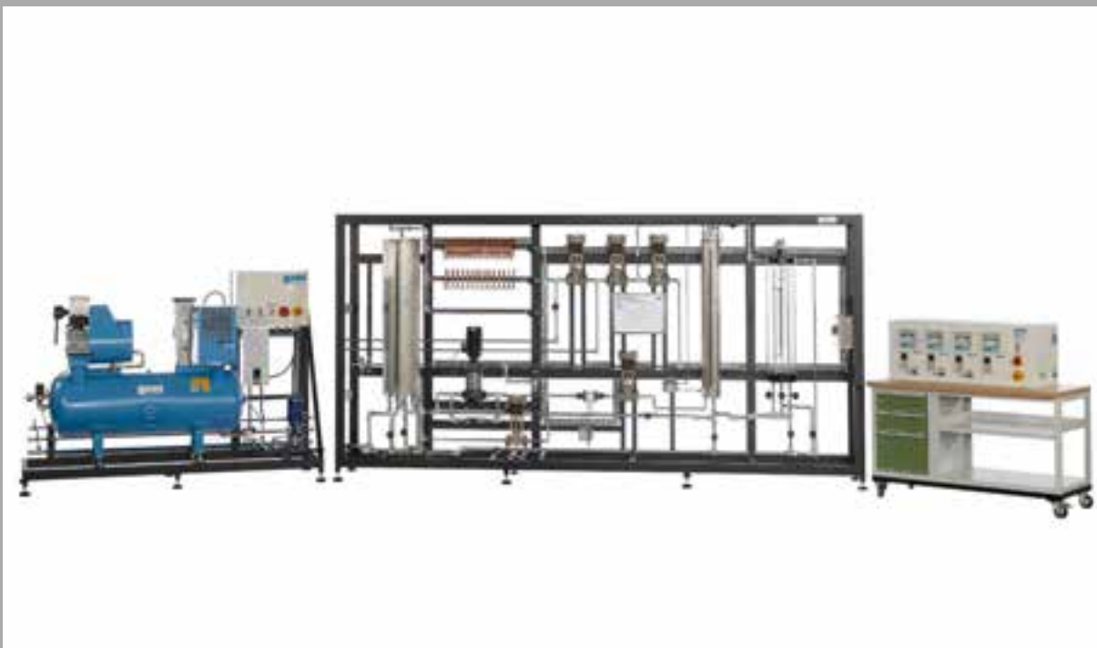
From left: supply unit, trainer and control station
