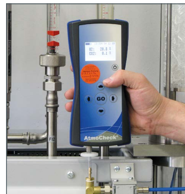
Gas analyser for determining the oxygen content and carbon dioxide content.
