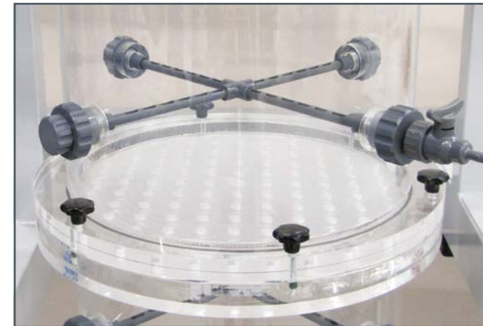
Sampling point within the trickling filter
